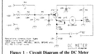
scale, or build a complete voltmeter by adding a 0-100  $\mu A$  meter.
