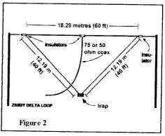
between 1000 and 2000 pF with a rated working voltage of 1 kV. The trap should resonate on 3,6 MHz.
